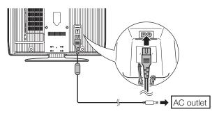
Place the TV close to the AC outlet, and keep the power plug within reach.
